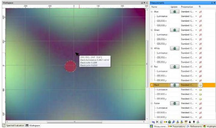
Photometrica® screenshot showing several measurement layers with luminance and x and y component layers. The Black layer is selected and RGB rendered in the Workspace. The cursor tooltip provides more detail.
