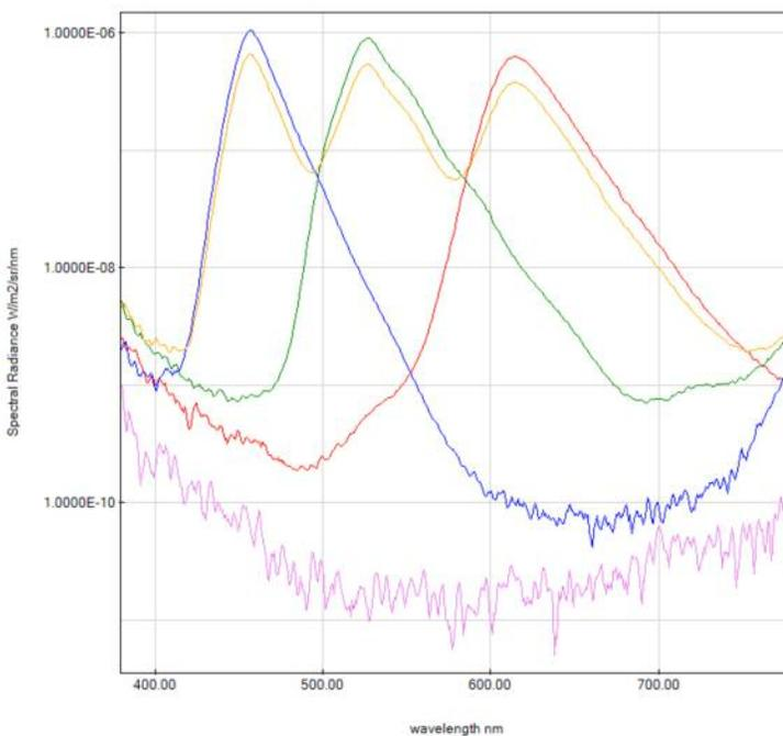
Red, green, blue, white and black OLED spectra measured by the WP214. For the blue OLED, the luminance is only 15 cd/m<sup>2</sup> and the peak is up to 5 decades above the instrument noise floor.
