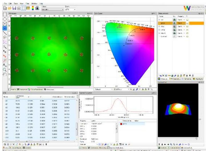
The results of a full analysis of a green emission source are displayed in the Photometrica® environment. Areas of interest, a line profile, surface plot, and 1976 u'v' color plot reveal the uniformity of the scene.
