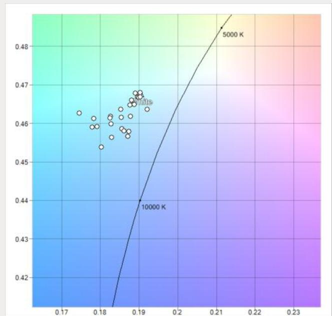
Examples of how the chromaticity varies at test points out to 50 degrees from the center for an OLED display set to blue, green, red and white.
