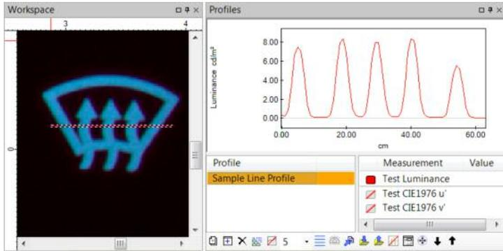
Photometrica® window shows an illuminated wall feature profiled at an angle.
