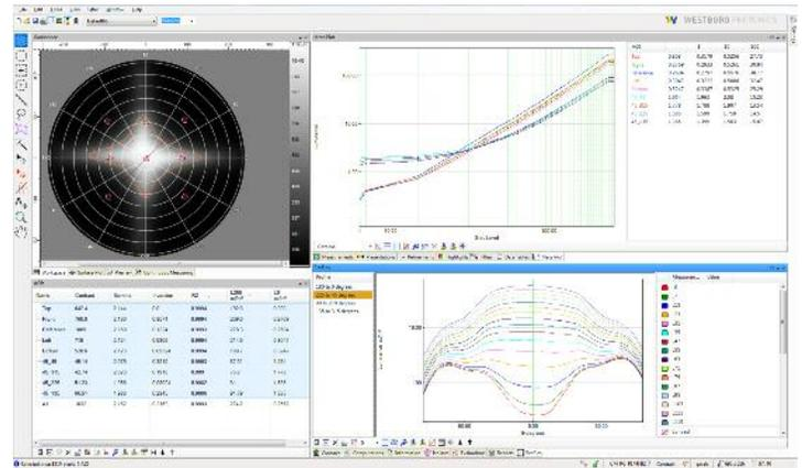
A series of measurements of the display luminance are taken from grey level "0" to "255". From the luminance measurement layers, derived layers of gamma, inversion and gamma fitting are created. The above screenshot of Photometrica® shows:
